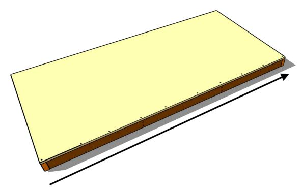
17. Once you complete the Stile side, go back to the point where you started and drive screws along the Rail, using the same method.
