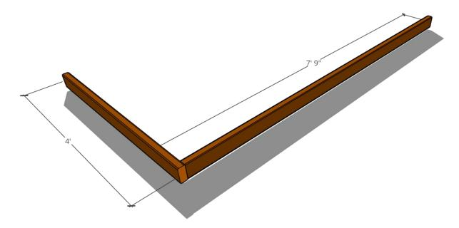
2. Apply glue to the end of the stile and press it into place against the rail. Ensure that the edges of the two boards are parallel and flush with each other. Using the ½" drill bit, drill two pilot holes through the Rail and into the end of Stile. Drive a 3" screw into each of the holes, tightening them until the two pieces of wood pull tight to each other.
