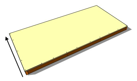
18. By now, the frame should be fairly rigid under the plywood. Work your way along the platform driving 2" screws along the Toggles one at a time, from the secured Stile side toward the unsecured Stile.
