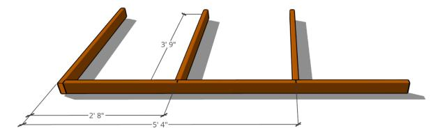
7. Place the second Rail at the exposed end of the Stile piece, and glue and screw it into place as you did with the first Rail in Steps 1 and 2.
