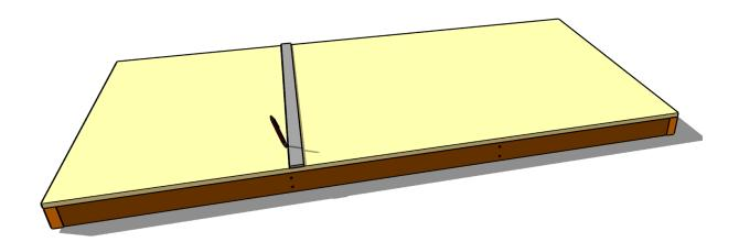
15. Beginning at one corner, make sure that the corner of the plywood and the frame underneath are squared up to each other. Don't worry too much about trying to get the whole frame squared up right away. Drive one 2" screw down through the plywood, driving it as close as possible to center on the frame (roughly ¾" from each edge). You do NOT need to pre-drill holes for these screws.
