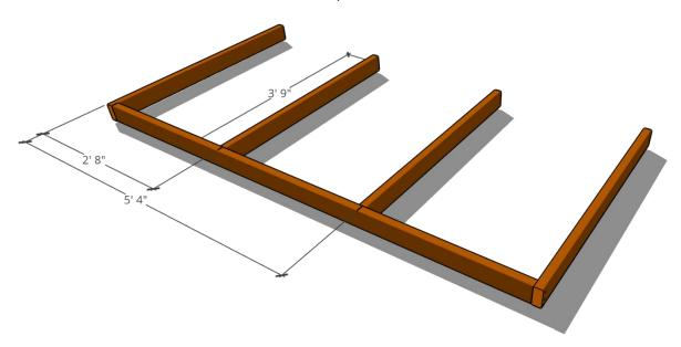
8. Place the other Stile on the open side of the frame and make the same centering marks on the Stile as you did in Step 3.
