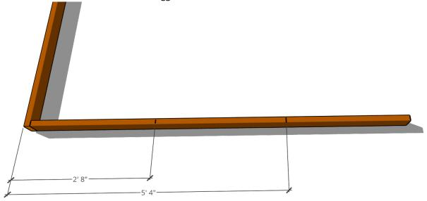
4. Starting at the 2' 8" (32") mark, place a Toggle (3' 9") on the "inside" of the Stile, so that it is centered on the mark you made.
