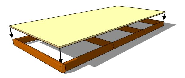
14. With a long straight edge and a pencil and using the visible screws along the stiles as your guides, draw lines across the face of the plywood to mark the center lines of the Toggles underneath. This will make it much easier to screw down through the face of the plywood into the Toggles later.
