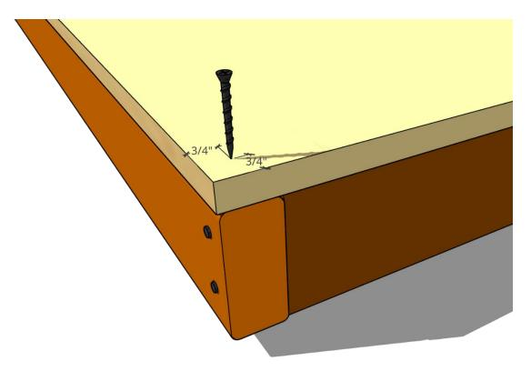
16. Working your way along the stile, place screws every 12" (You do not need to predrill these). Pay close attention to the plywood and the Stile as you do this, they should be flush at the point where you're screwing each time. You can easily shift the frame or the plywood back and forth slightly as you go to make sure that they are being joined as evenly as possible.
