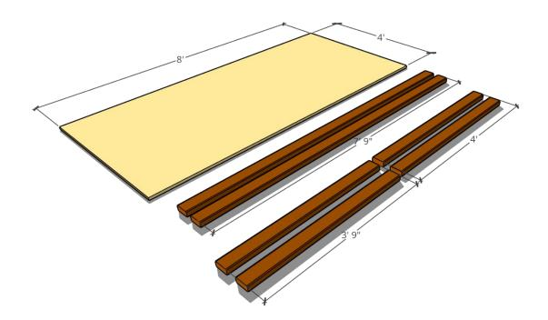
Note about cutting boards to length: When cutting you must account for the Kerf (width) of the saw blade you are using. For example, this means you cannot cut two 4' lengths from an 8' board, because one of the boards will wind up slightly shorter than 4' long.
