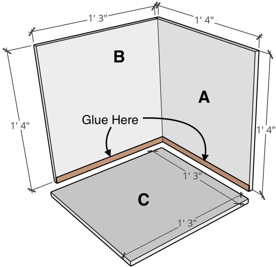
4. Staple through the outsides of panels A and B into the edge of panel C. If you have a reliably flat work surface, you can move the piece to the edge of your surface and use it as a guide to ensure that the pieces remain properly flush while stapling. If not, I would recommend rotating the piece as you work so that you have a clear view of how the panels are lining up as you attach them to each other.
