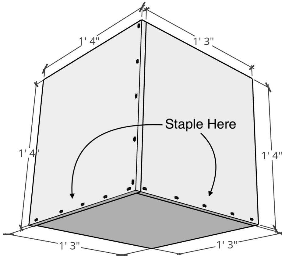
6. Glue along the exposed edges of the box, and place and staple the final panel A piece into place.
